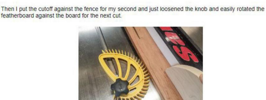
The featherboard can be re-configured to use on the left or right side of the fence. There is also an
